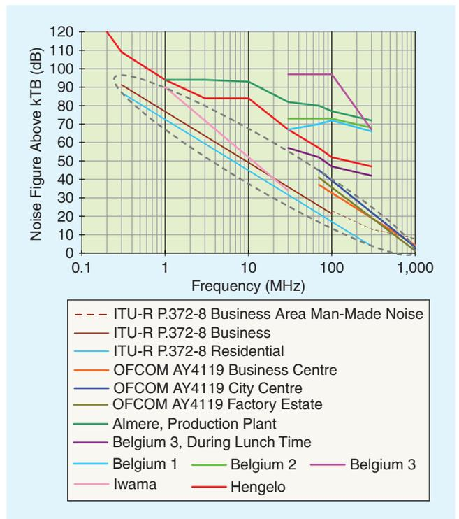
Fig. 2. Noise levels outside buildings and in semi-enclosed, industrial, environments. The lines within the ellipsoid are the noise levels outside buildings.
